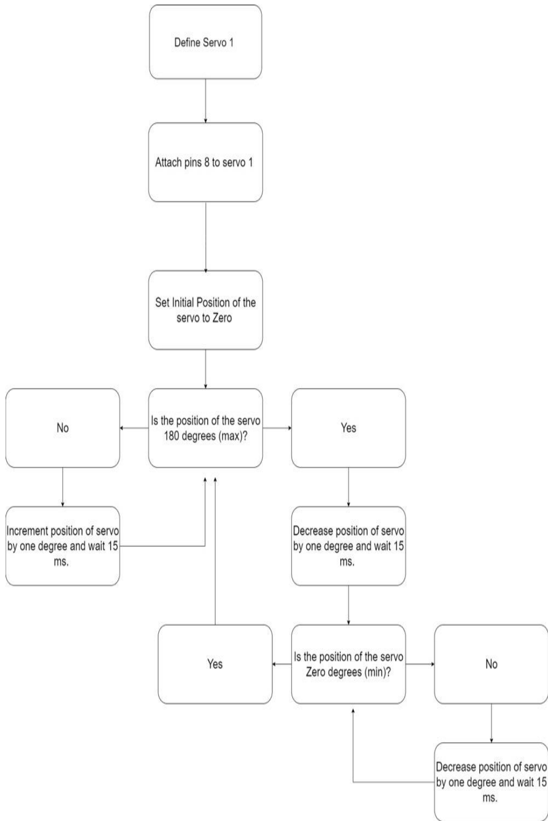
Figure 6.17 Fifth Code Diagram Sweeping code for calibrating the servo motors
